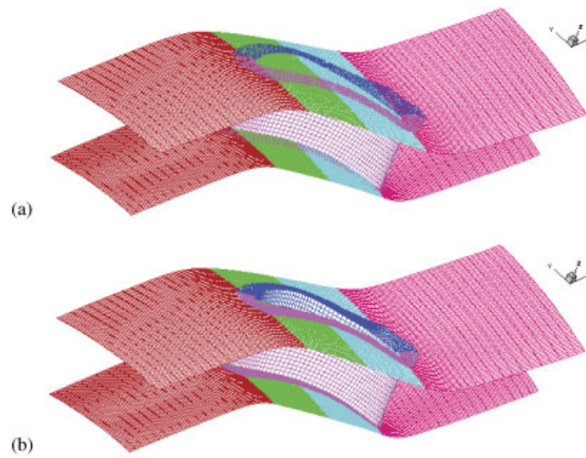
Figure 12. The overset grid for a turbine stator: (a) before implicit hole cutting and (b) after implicit hole cutting.
